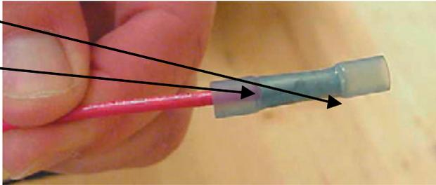
4. If desired, use a heat source to seal the splice, being careful not to damage the wire insulation. You want to insure that the wire installation has no signs of overheating or mechanical damage.
