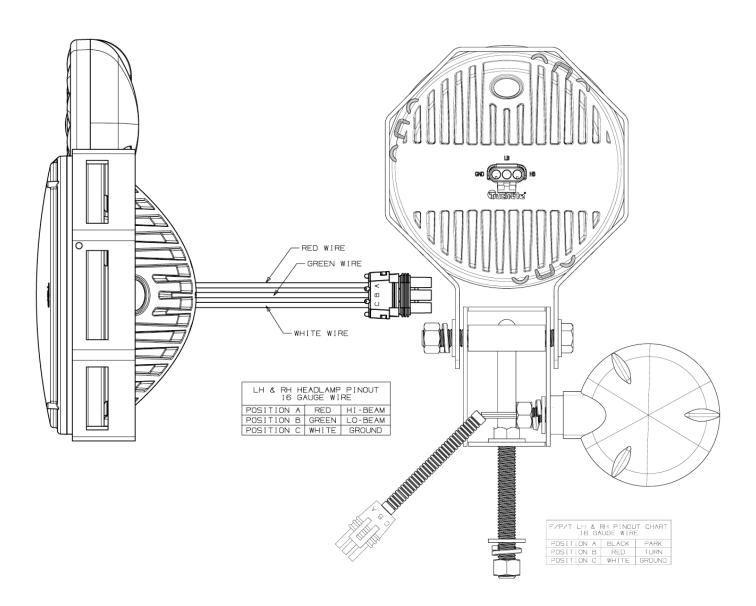
Truck-Lite's 7-inch Round LED Snow Plow Kits are designed for use with a snap-together harness (80898). If wiring directly to vehicle power\*, use the details below to determine the appropriate wire for each function.
