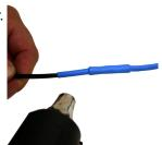
allow its casing to seal the connection.
