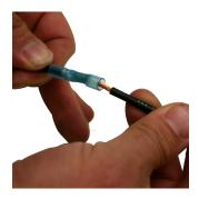
important that the insulation does not extend into the crimp and that the wire is clean and bright.
