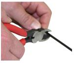
The cut and stripped wires should be clean and bright.
